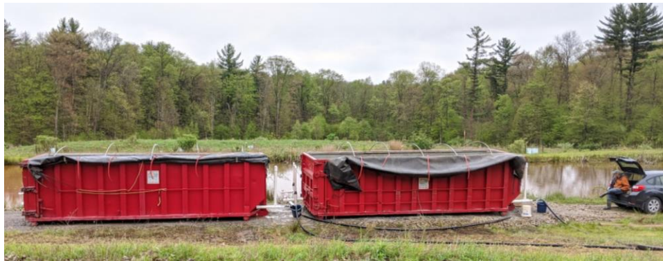
Pilot-scale limestone-filled containers used for CaCO 3 +CO 2 experiments.
